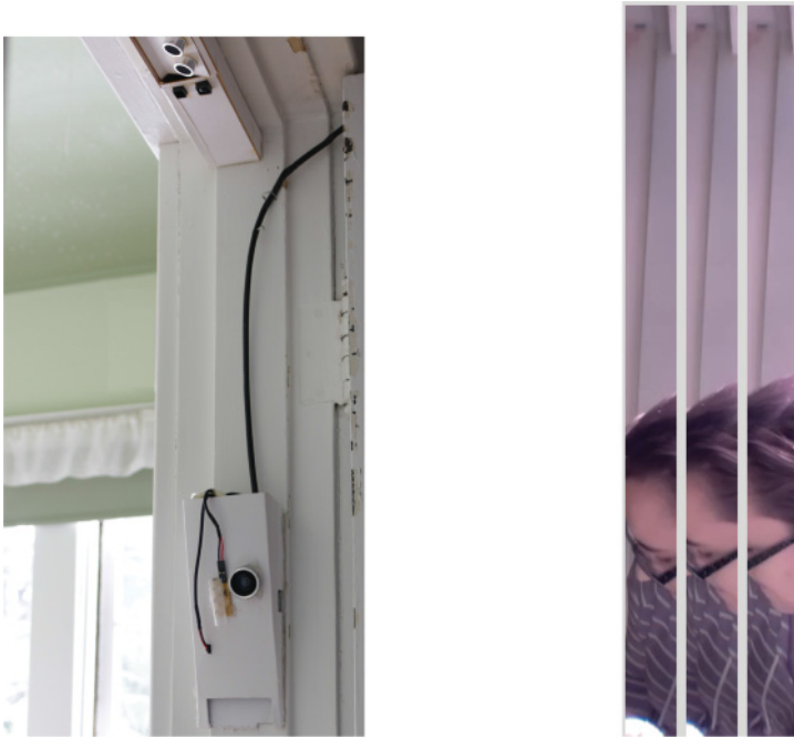
Fig. 7. The cameras (left) were placed in each doorway to record a narrow video (right) of only the doorway interior. This was used for ground truth detection of when people crossed between rooms.
