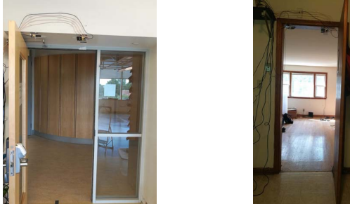
(a) Doorpler was mounted atop an office doorway. A scripted study and an 80-hour in-situ study was performed on this doorway yielding over 1500 doorway crossing events. (b) Doorpler was mounted atop the most commonly used doorway in a 2-person home for 120 hours yielding 113 doorway crossing events.
