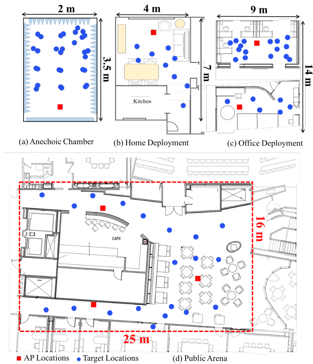
Figure 5: Experiments were run in four environments with varying size and multipath complexity. The closest AP to each target was used for localization.
